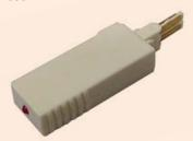
Single Line Arrestors are used to protect modern telecommunication equipments from damage caused by transient surge voltage, over single pair cable in MDF Frames or distribution box. Protection unit is made of ceramics gas discharge tube. Overcurrent protection is also available with ceramic gas discharge tube with additional "Fail Safe Mechanism".
